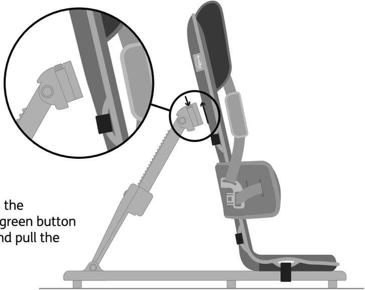
To release GoTo from the floorsitter, press the green button on the recline arm and pull the back rest forward.
