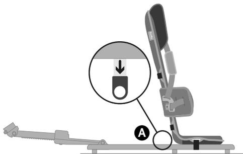
To release the seat base, pull on the green plastic tab **A** and slide backwards, then lift GoTo off the floorsitter. **B**
