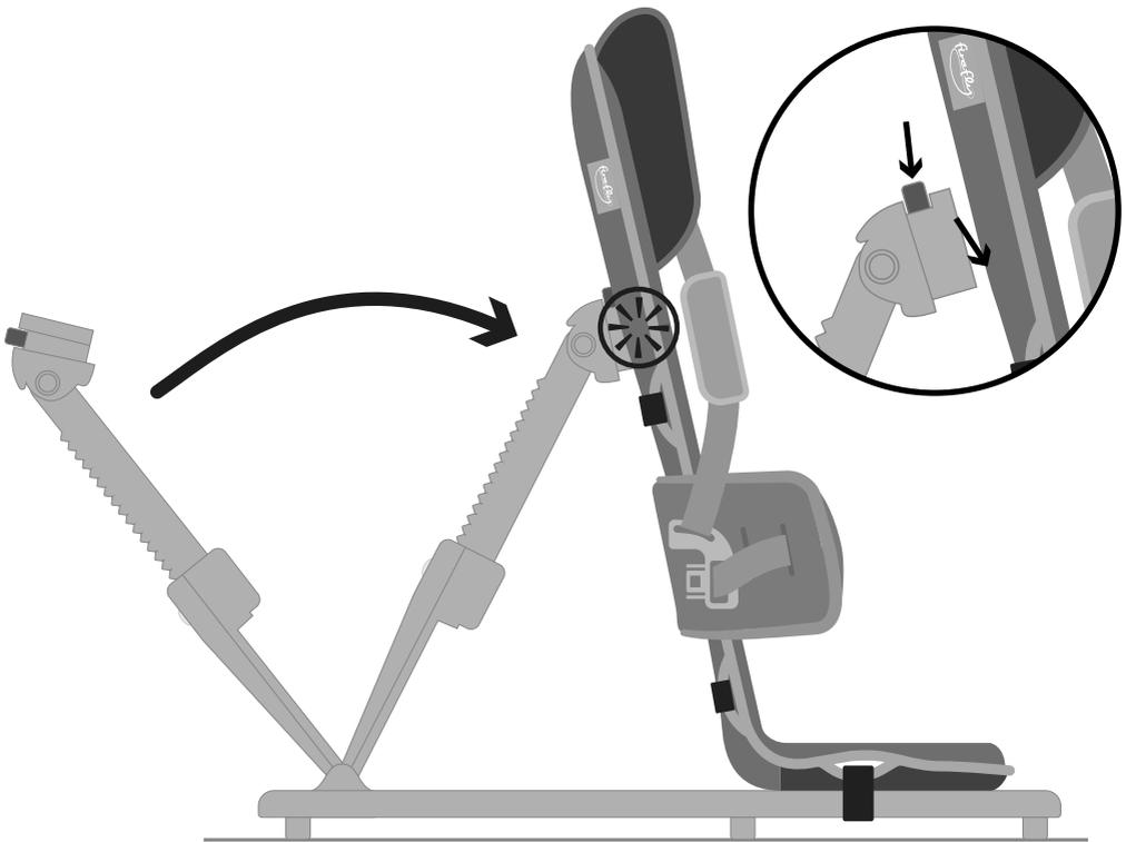
Before attaching the recline arm to the backrest, ensure that it is at the highest setting.
