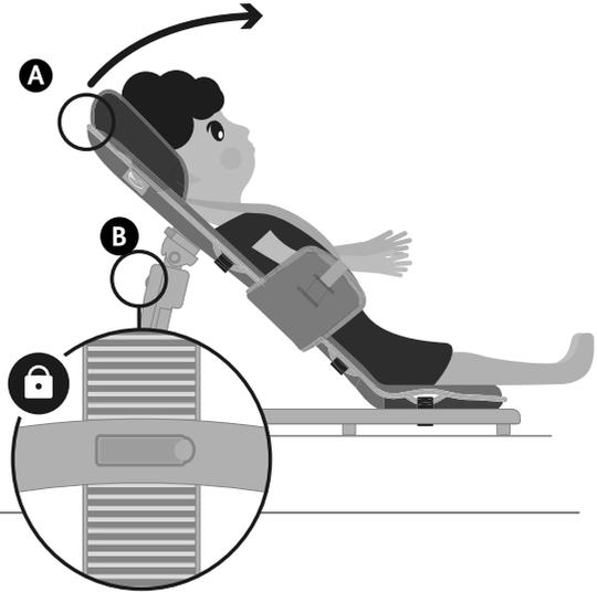
Release the clip and bring the seat into an upright position that is suitable for your child. **A**
